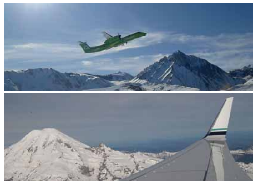
Above: Flying on a Horizon Air Bombardier Q400 turboprop, affectionately known as a "Green Machine," is roughly equivalent to driving in a car that gets 64 miles per gallon. A Q400 is 30% to 40% more efficient than a comparable-sized jet. Below: Alaska Airlines is using winglets, like the one shown here, to further increase aircraft fuel efficiency by 3% to 5%. That translates into approximately 100,000 fewer gallons of fuel consumed per aircraft each year.
